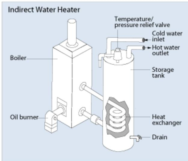
Indirect systems can be fired by gas, oil, propane, electric, solar energy, or a combination of any of these. Tankless systems are typically electric or gas-fired. Also, these integrated or combination water heating systems not only can work with forced air systems but also with hydronic or radiant floor heating systems.
