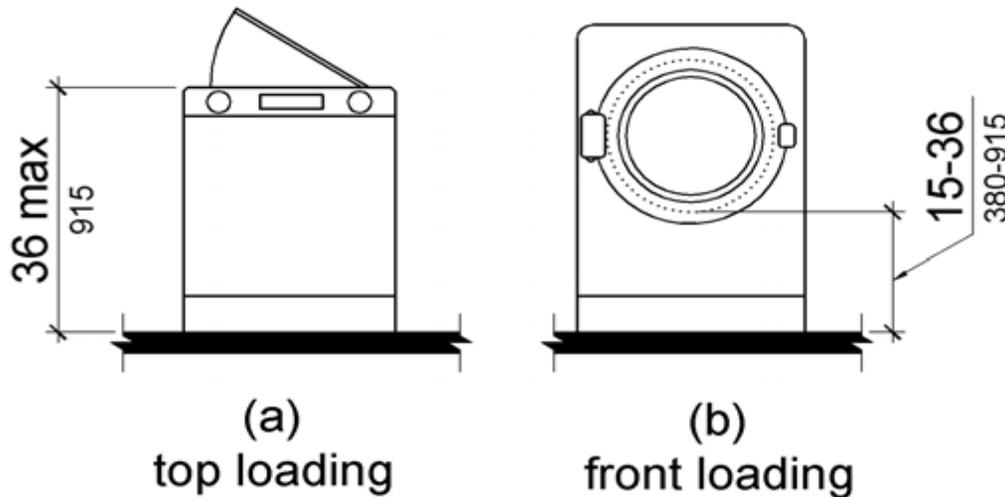
**Figure 611.4 - Height of Laundry Compartment Opening**
