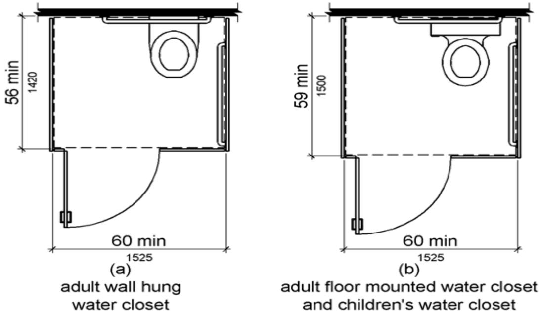
**Figure 604.8.1.1 - Size of Wheelchair Accessible Toilet Compartment**
