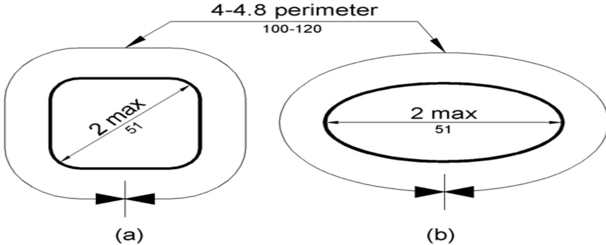
**Figure 609.2.2 - Grab Bar Non-Circular Cross Section**
