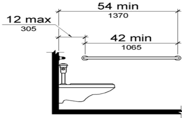
**Figure 604.5.1 - Side Wall Grab Bar at Water Closets**
