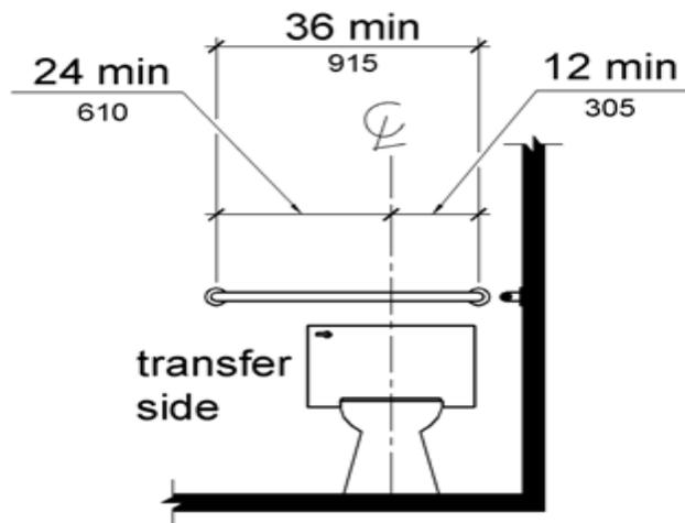
**Figure 604.5.2 - Rear Wall Grab Bar at Water Closets**
