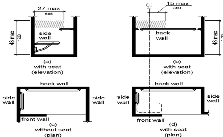
**Figure 608.5.3 - Alternate Roll-In Type Shower Compartment Control Location**
