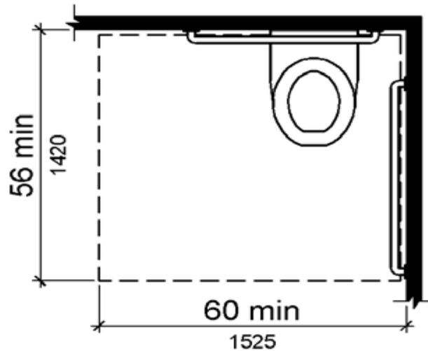
**Figure 604.3.1 - Size of Clearance at Water Closets**
